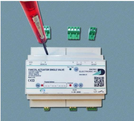
Remove the terminal cover with a screwdriver
